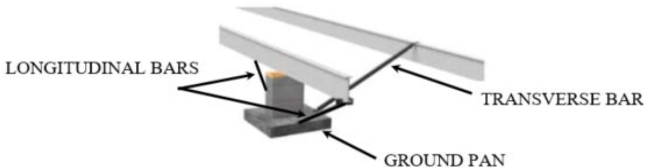
Figure 20. Typical installation of a Ground (Pan) Foundation System
