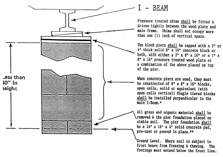
Pier foundations shall be installed directly under the main frame (or chassis) of the mobile home. The piers shall not be further apart than ten (10) feet on centers on the main frame, front or back, and shall not extend further than five (5) feet beyond the center line of the end of the piers.
